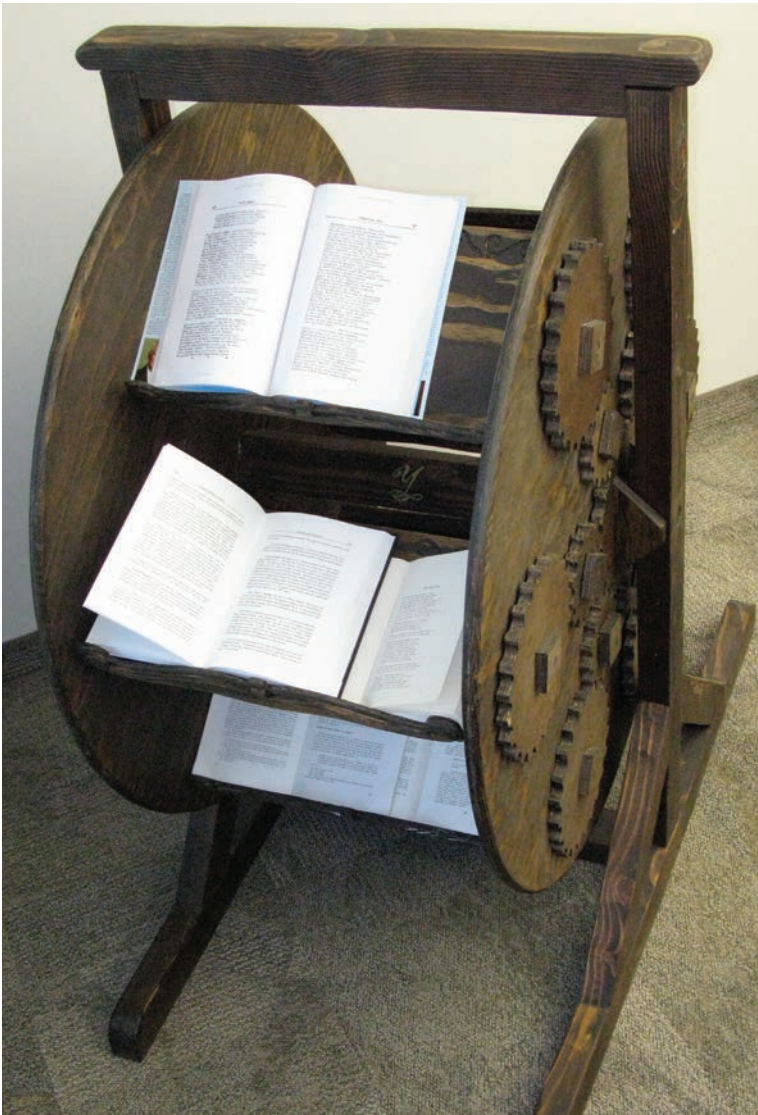
Facsimile of a book wheel constructed by Jason Yancey (MA 2005) after Ramelli's design
